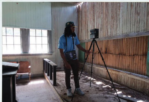
John Richardson conducting 360 photogrammetry at Mt. Olive. (NCPTT)
